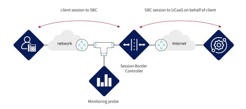
UC clients, either remote or connecting through an enterprise network connect to a Session Border Controller (SBC) which hides the network topology and protects the service provider or enterprise packet network.
