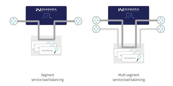
A single segment can be protected by multiple servers for increased service availability and resilience. Combining multiple segments protected by security services provided through multiple servers (COTS) allow for advanced service protection and optimized server deployments.
