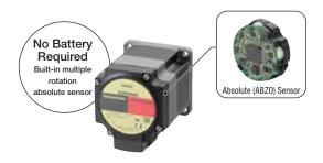
The AZ Series is a "hybrid" stepper motor-based motor & driver system that combines the advantages of the "open loop" set up programming with "closed loop" performance. In addition to high-accuracy positioning and speed control, it can perform control that restricts the motor's generated torque to a set value for push-motion operation.
