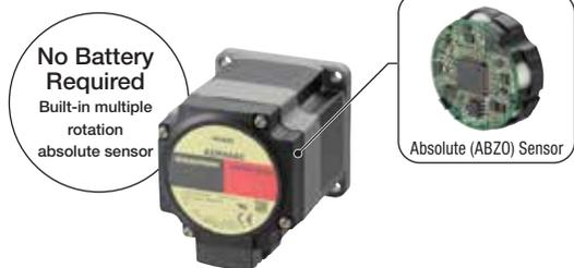
The AZ Series is a “hybrid” stepper motor-based motor & driver system that combines the advantages of the “open loop” set up programming with “closed loop” performance. In addition to high-accuracy positioning and speed control, it can perform control that restricts the motor's generated torque to a set value for push-motion operation.
