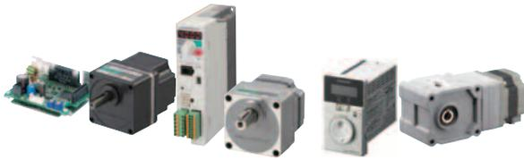
Brushless motors offer excellent energy efficiency and savings equivalent to IE4, excellent speed stability, as well as a wide speed control range. Brushless motors use permanent magnets in the rotor of three-phase motors. With Brushless motors there is no brush and commutator resulting in a maintenance free motor.
