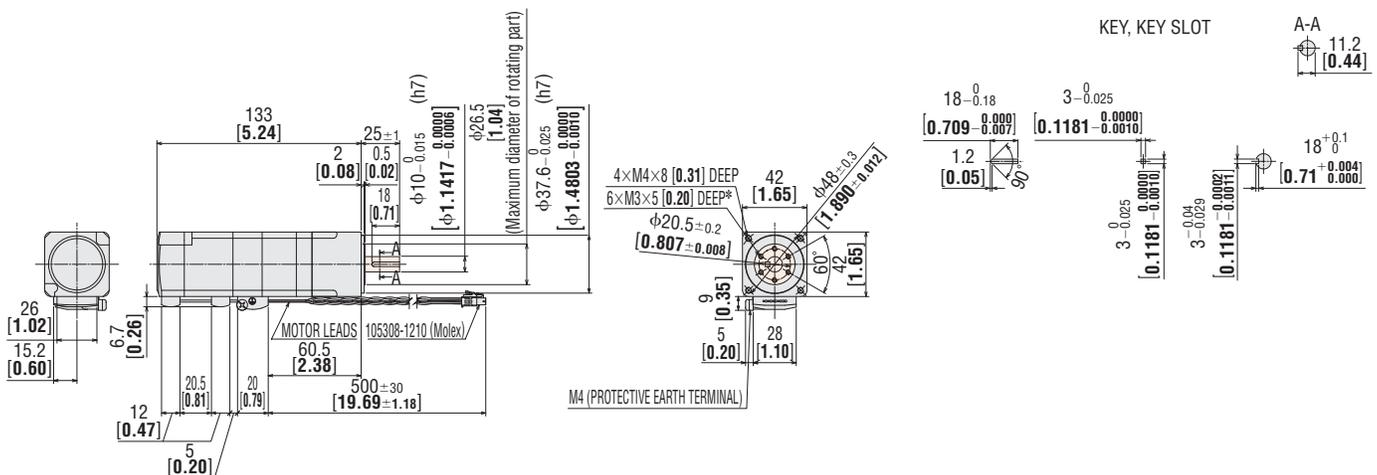
\*The position of the output shaft relative to the screw holes on the rotating part cannot be specified. Adjust the position via the size of the screw holes on the load installation surface.
