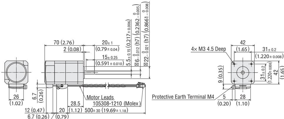
◇ Standard Type with an Electromagnetic Brake
