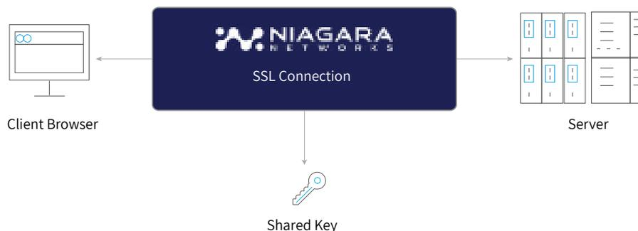
*With PFS, unique session keys are generated using both client and server information. The challenge that PFS presents is that PFS handshakes are incompatible with the decryption capabilities in network monitoring tools which analyze network traffic.*
