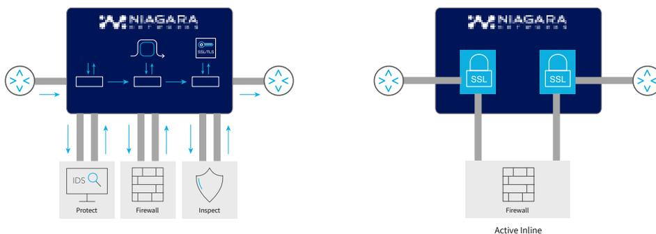
With Active-Inline decryption the received traffic is, after optional pre-filtering, sent to the decryption engine. After decryption, the traffic is forwarded to the inline appliance. The packet brokers service chaining capabilities enables cascading of multiple inline security appliances, all receiving the decrypted traffic. If one of the protections appliances in the chain would unexpectedly fail, the packet broker bypasses the failed appliance thereby restoring the security chain.
