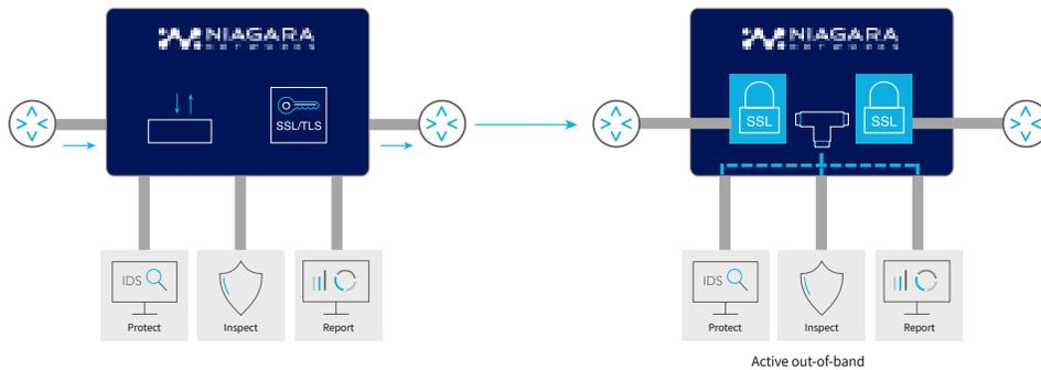
The received traffic is decrypted, and a copy of the decrypted traffic is sent to the inspection and reporting tools. After copying, the traffic is immediately re-encrypted and forwarded for further processing.
